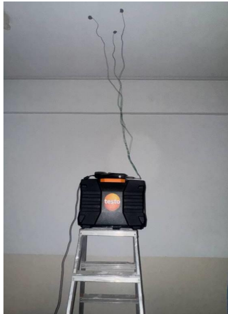
Figure 6: Experimental setup for U-value measurement of the ceiling using external sensors.
